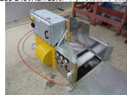
Charging Station (Contactless Charging and re-purging)
